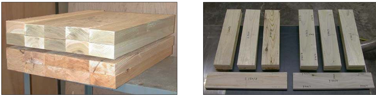
Figure 3.1. The machining of the wood samples: timber (left), lamellae (right).
