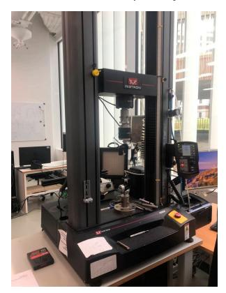
Figure 2. Instron 5969 Dual Column Testing System with material Glycolon in vise.
