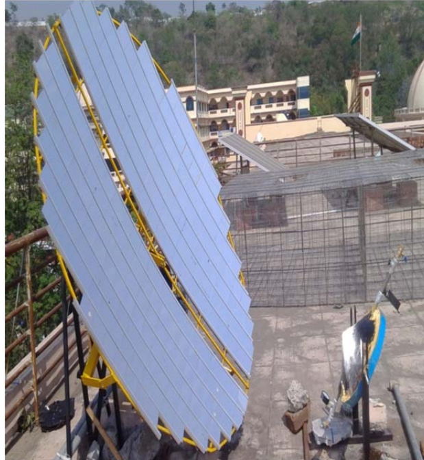
Fig.1. Experimental setups ( tilt condition) of small Scheffler ,concentration ratio 17 with conical receive
