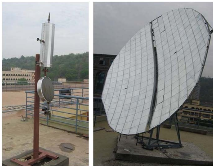
Fig.2. Experimental setup (Normal condition) of big Scheffler, concentration ratio 48 with cylindrical receiver
