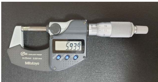
Figure 3. Measure the length of the specimen using a digital micrometer.
