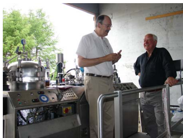
A compact continuous extraction facility using HFC-134a. (Peter Wilde Associates Ltd.)
