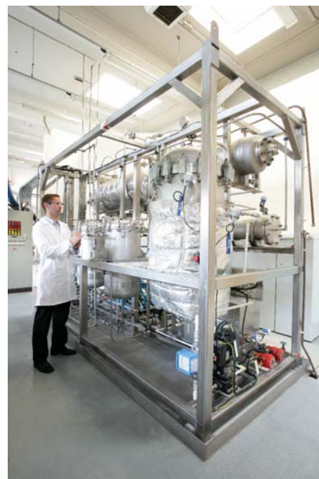
Pilot plant for continuous extraction using HFC-134a at Ineos Fluor Ltd.
