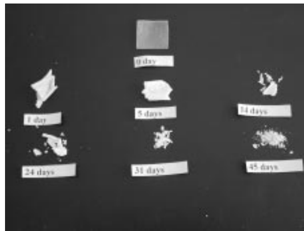
Fig. 5 Evolution of the physic state of the PLA film pieces during their degradation in liquid medium according to the 14852 ISO/CEN norm.
