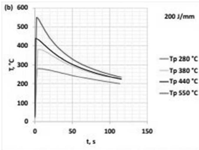
**Figure 5.** HAZ thermal cycles at high heat input (200 J/mm)
