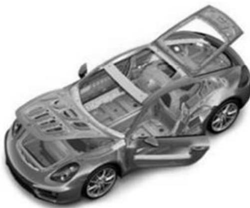
**Figure 2.** High strength aluminium alloys in a sport car-body [21]**Slika 2.** Aluminijumske legure visoke čvrstoće u karoserijama sportskih automobila [21]
