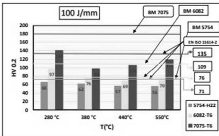
**Figure 8. Hardness distribution in HAZ at different linear heat inputs**
