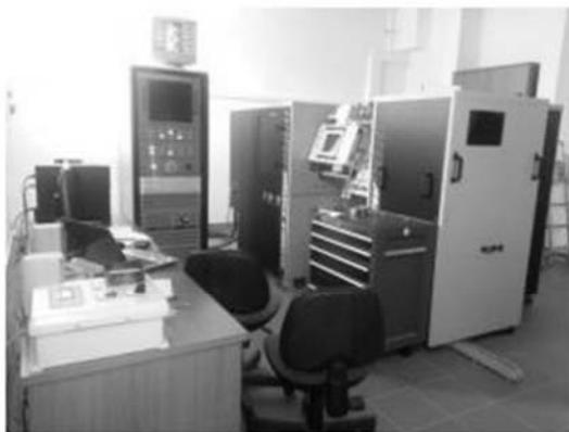
**Figure 3. Gleeble 3500 simulator system**
