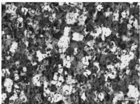
**Figure 10 (a)**  $T= 550^{\circ}\text{C}$ , Linear heat input  $200\text{ J/mm}$
