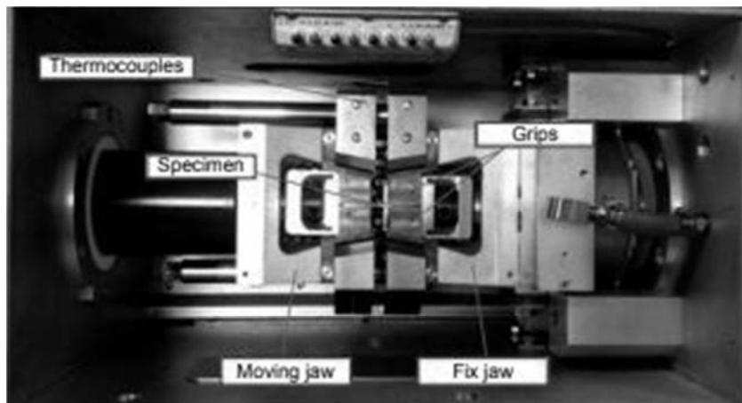
**Figure 7. Specimen in the test chamber**
