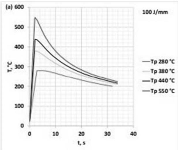
**Figure 4.** HAZ thermal cycles at low heat input (100 J/mm)
