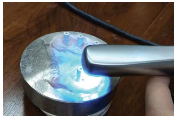
Fig. 1. Scanning the master model with the intraoral camera (True Definition, 3M ESPE).
