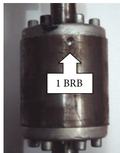
FIGURE 5: One broken rotor bar.
