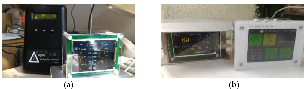
Figure 1. Pictures of the Dylos air quality monitor and a GPM sensor without housing at the background site (a) and a GPM sensor with aluminum housing next to a BH1 unit at the urban site (b).
