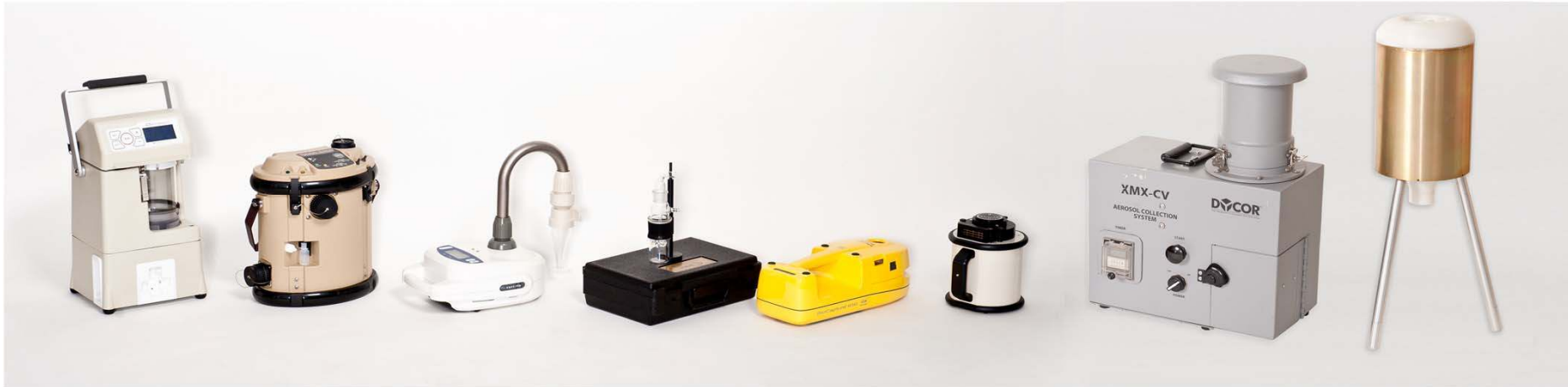
Figure S2. Air sampling equipment subjected to testing and evaluation (T&E) in this study. From the left: OMNI-3000, SASS 2300, Coriolis FR, BioSampler (reference sampler), BioCapture 650, SASS 3100, XMV-CV, and ESP (prototype). The gelatin filters are not shown in this picture.
