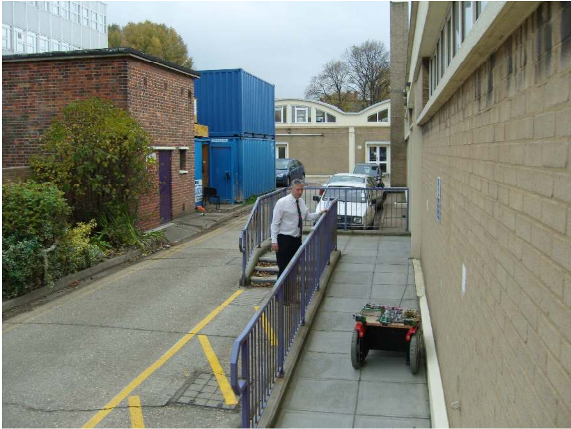
Figure 6 View observed by a tele-operator in a laboratory from an external camera while driving the robot through a complicated outdoor environment using an umbilical cable and assisted by the sensor system.
