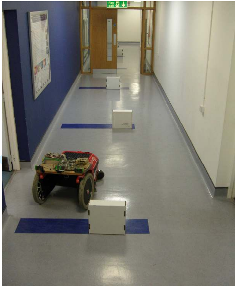
Figure 3 Radio controlled robot moving through a complicated corridor assisted by the sensor system on the mobile-robot.
