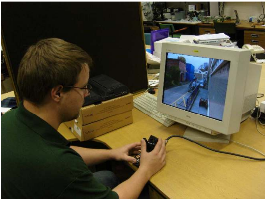
Figure 2 A tele-operator in a laboratory controlling the robot through an umbilical cable with a camera set up to observe the environment and the robot.
