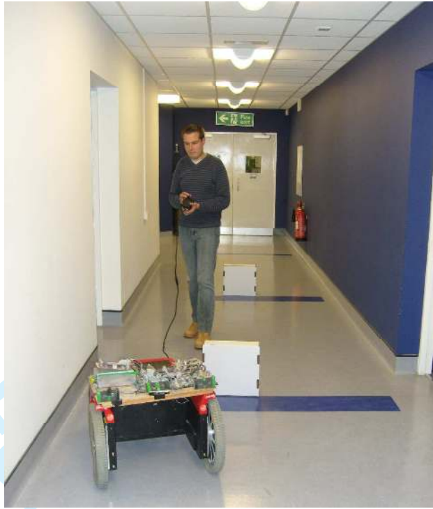
Figure 1 Tele-operator navigating through one of the complicated corridors using the ultrasonic sensor system to assist in steering.
