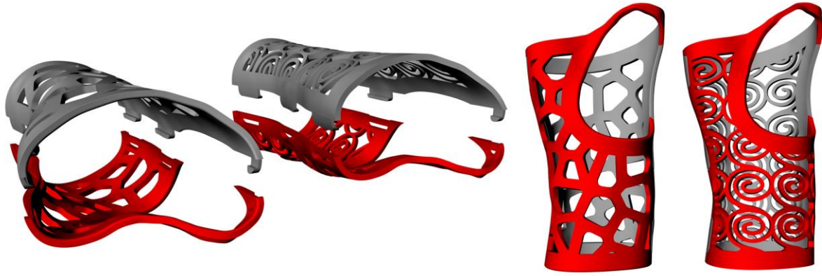
Figure 4: Circumferential, homogeneous two-part splints for SLA (Voronoi) and Objet ('Swirl') builds respectively
