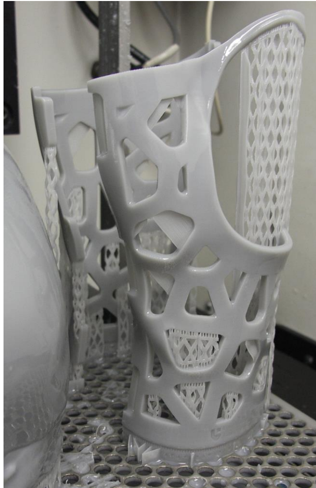
Figure 9: SLA build, showing support lattice structures. Image courtesy of S. Peel at PDR, Cardiff
