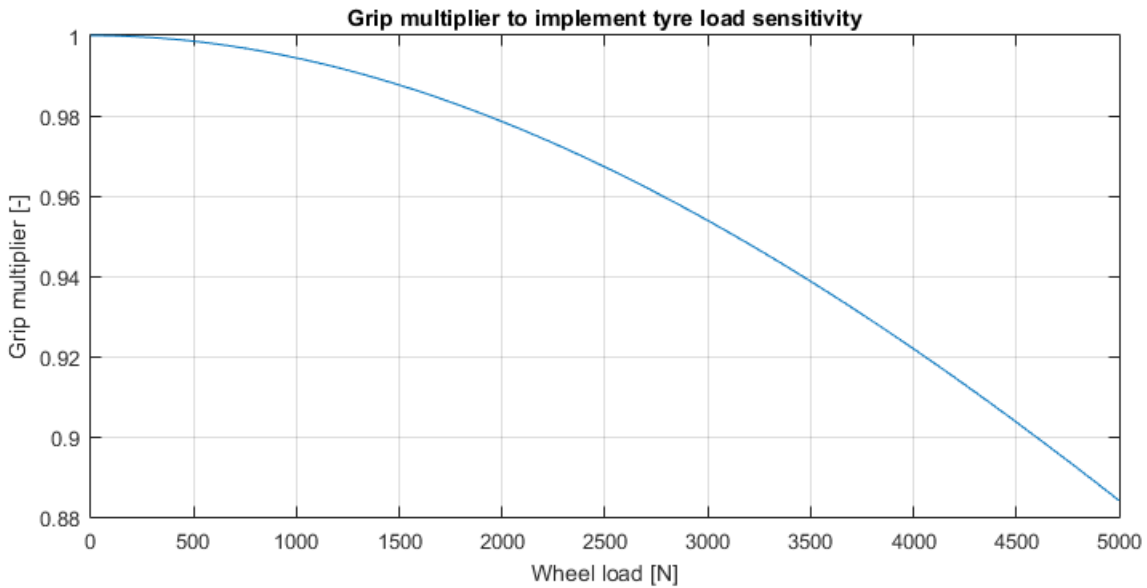
Figure 4.1: Modelation of tyre load sensitivity in rFactor, decreasing grip with increasing tyre load.
