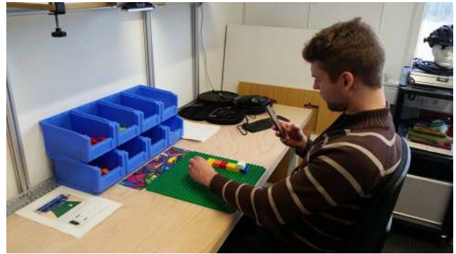
Figure 4: Smartphone providing in-situ AR assistance
