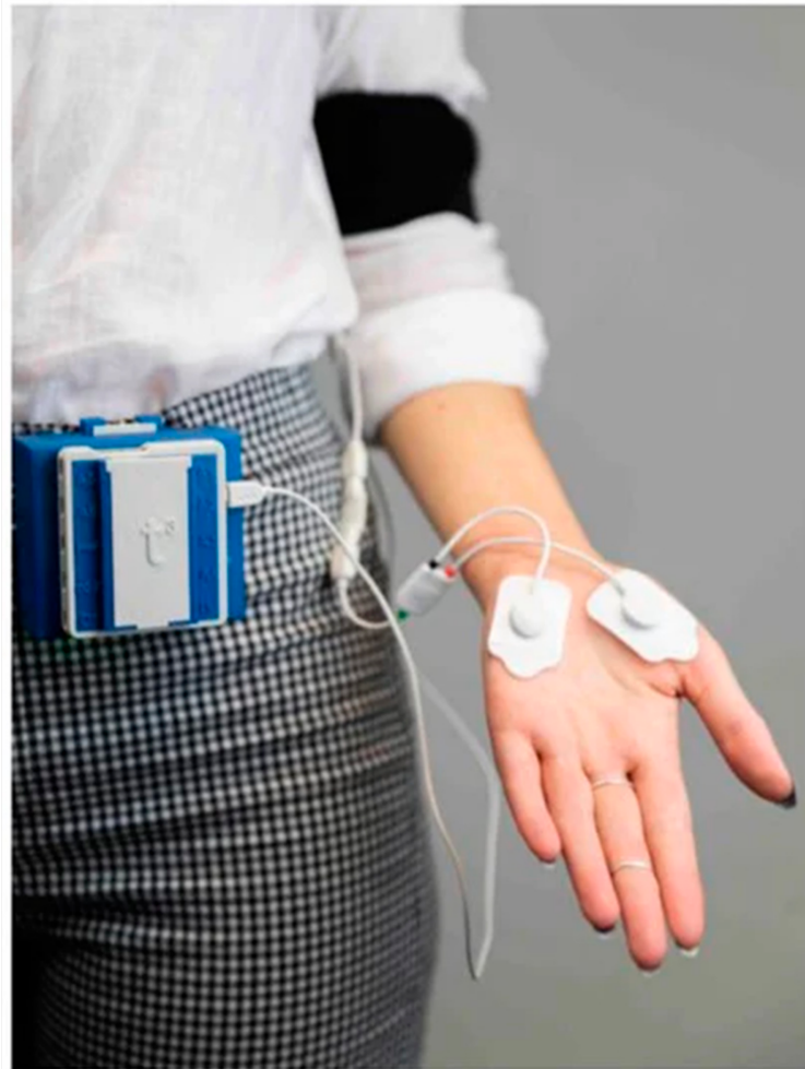
Figure 3. The electrodes placed on the participant's non-dominant hand are connected to sensor cables wired to the COBALT Bluebox device. Image source: Brissette-Gendron, R., Léger, P.M., Courtemanche, F., Chen, S.L., Ouhana, M., and Sénécal, S. (2021). The response to impactful interactivity on spectators' engagement in a digital game. Multimodal Technologies and Interaction , 4(89), 89–89. https://doi.org/10.3390/mti4040089 , accessed on 20 December 2021.
