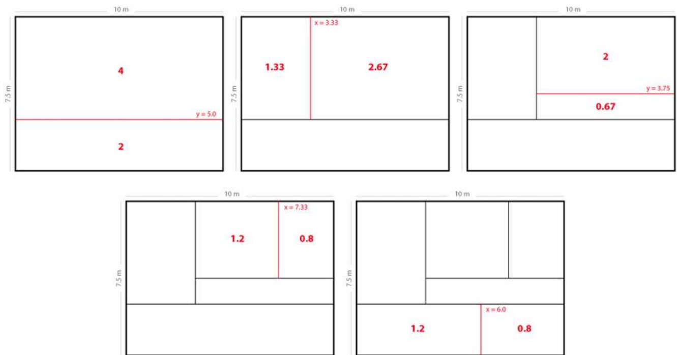
Fig. 2. Subdivision sequence and geometrical ratio in a layout. Syntax: H(V(o)(H(V(o)(o)(o)))(V(o)(o))). Reprinted with permission from Knecht and Koenig (2012).
