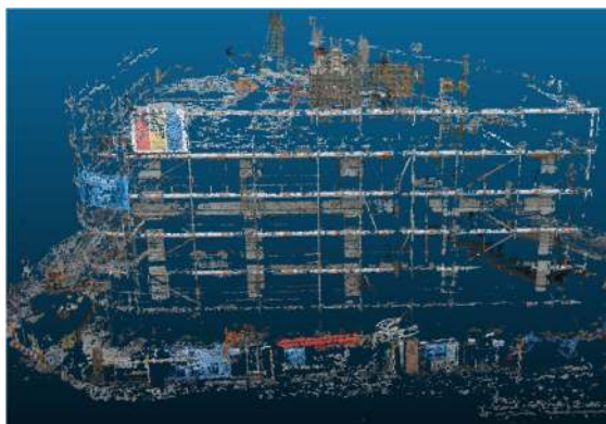
Figure 7. Dense point cloud created from the images shown in Figure 6.
