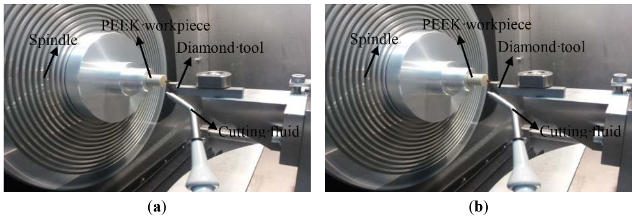
Figure 3. Main sections of the cutting process (a) PEEK; (b) PEEK CF 30.
