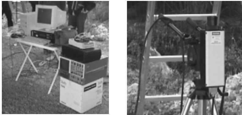
Fig. 4. Laser Doppler vibrometer measurement head and chain.
