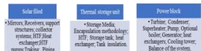
Fig. 1. Components of CSP plant [10].
