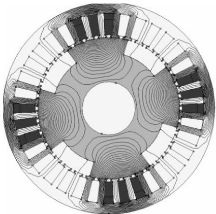
Fig. 12. Flux distribution in q-axis.
