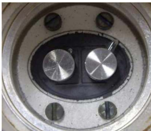
Figure 1. The glass capillary vessel that was inserted into an aluminum holder.
