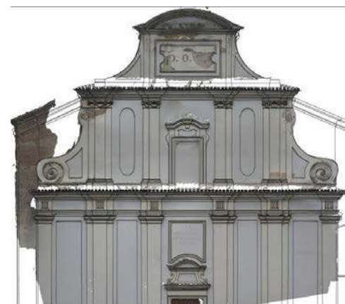
Figure 8: Comparison between the ortho-images of the façade and the digitalization obtained from the scanner point cloud.
