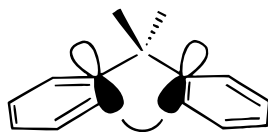
Figure 9. Through-space overlap of p atomic orbitals of diphenyldimethylsilanes and 2,2-diphenylpropanes in a butterfly conformation.
