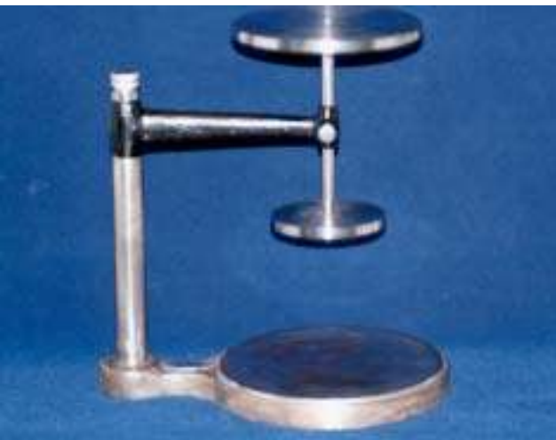
Fig. 3 – Device to uniform the load (kg) applied over the models.
