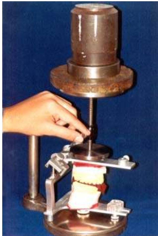
Fig. 5 – Carbon paper interposed between the models mounted in articulator submitted to a load of 10 kg to record the occlusal contacts.
