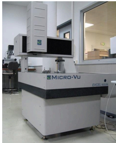
Figure 3: CMM of the type MICROVU EXCEL502UM placed at LNE.
