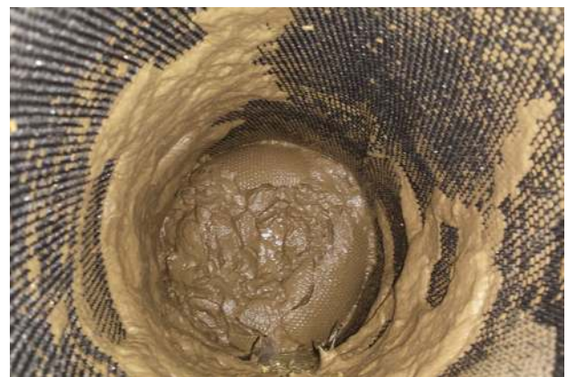
Fig. 9 Filter cake after first filling in 2-D test
