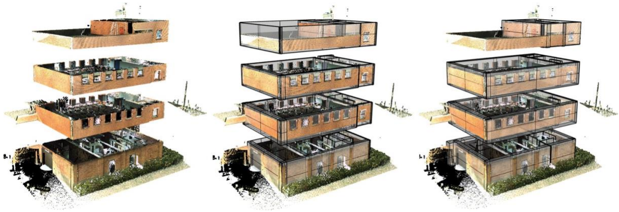
FIG. 11: Overview reconstruction results. The initial point cloud (left), the reconstructed geometry by the 3D method (middle) and the reconstructed geometry by the 2D method (right).
