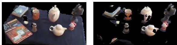
Figure 10: Point cloud before (left) and after (right) the persistent features computation
