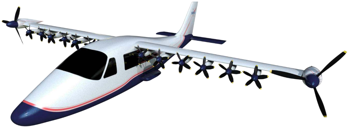
Figure 1: NASA's X-57 "Maxwell" Distributed Electric Propulsion Flight Demonstrator (Mod 4 Configuration)
