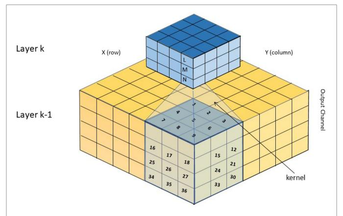
**FIGURE 1** | Schematic of a convolutional neural network, showing two layers. Each layer consists of multiple 2-D planes of neurons, one layer per output channel (feature). A given neuron on layer k receives input from a patch of the layer below, each input weighted by a set of kernel coefficients. The same set of coefficients is typically shared by every neuron on the same layer, although different output channels have distinct kernels.
