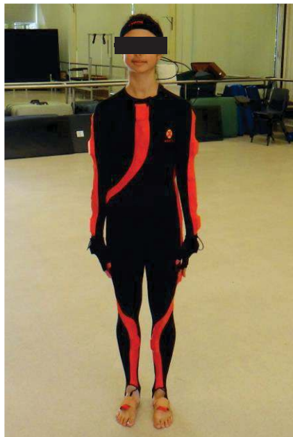
Figure 3. 2 Illustration of the participant during the static calibration with the MVN Xsens suit
