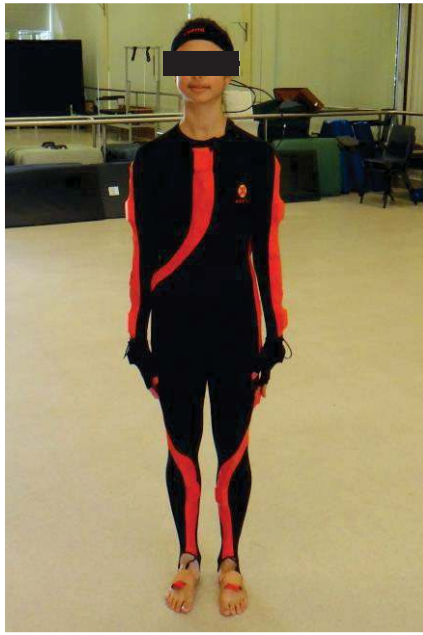
Figure 4. 1 Illustration of the participant during the static calibration in the MVN Xsens suit
