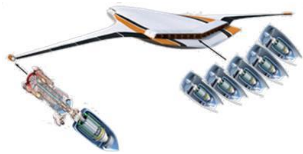
Fig. 1: NASA N3-X TeDP aircraft with wingtip mounted generators and propulsors along aft of the aircraft
