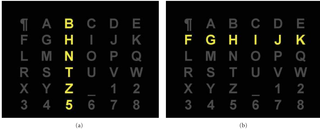
FIGURE 2: Typing matrix of the P300 speller. Rows and columns are intensified in random order; one trial consists of the intensifications all six rows and all six columns. The intensification of the third column (a) and of the second row (b) are shown.
