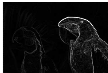
(f) Sobel filter output on the R - G plane
