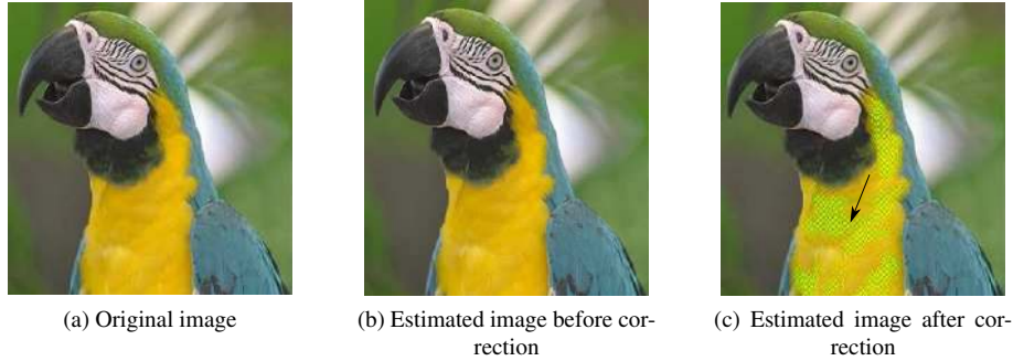
FIG. 21: Demosaicing result achieved by Kimmel's method (1999), before and after the iterative correction steps. Generated artifacts are pointed out on image (c).
