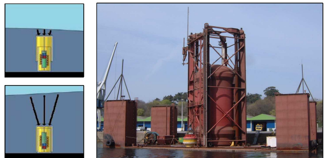
Fig. 1. The AWS working principle and the first prototype before submersion
