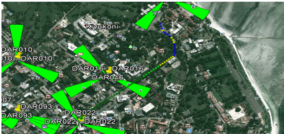
Figure 3: Drive test simulation in urban area Dar es Salaam
