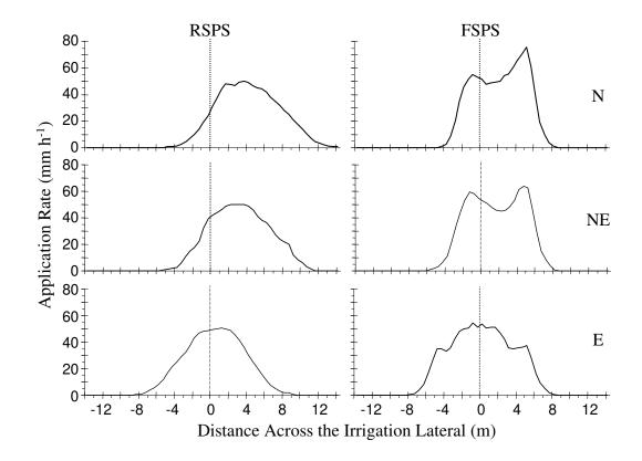
**Figure 11**. Wind speed effects on the OWEDL for the FSPS and RSPS.
