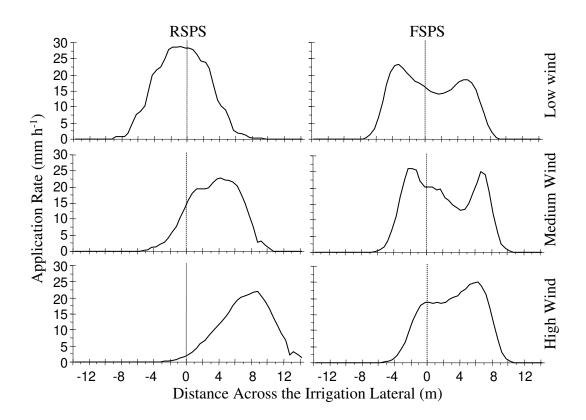
**Figure 10.** Simulated cross-sectional water distribution (mm h<sup>-1</sup>) of an irrigation lateral with 3.5 m spacing, a nozzle diameter of 6.7 mm, a spray sprinkler height of 1.0 m and high wind speed, for RSPS and FSPS and wind directions N, NE and E.
