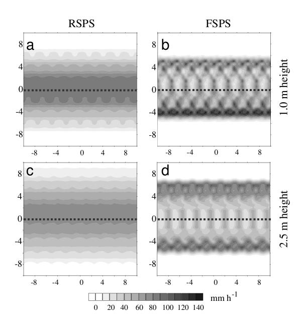
**Figure 8.** Simulated cross-sectional water distribution (mm h<sup>-1</sup>) of an irrigation lateral with 3 m spacing under low wind speeds and a spray sprinkler height of 1.0 m for RSPS and FSPS, and for the three nozzle diameters.
