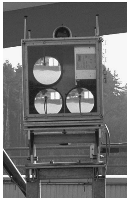
FIG. 1. Receiver of PSI's scintillometer showing the three-mirror configuration for the simultaneous measurement of horizontal and vertical crosswind.
