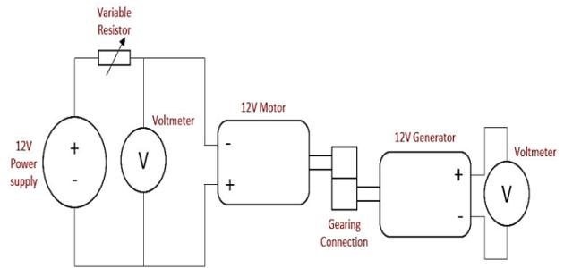
Fig. 4: Generator without load test wiring diagram
