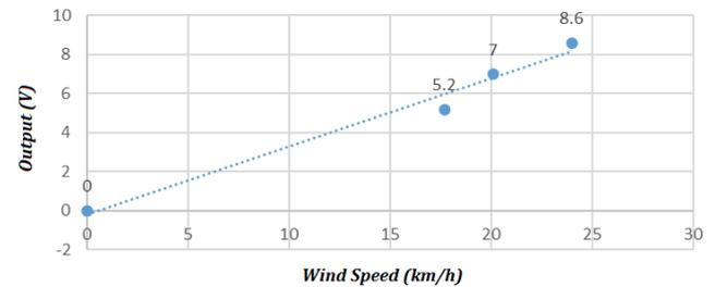
Fig. 14: HAWT indoor testing without load
