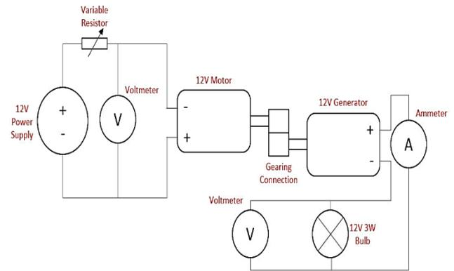
Fig. 5: Generator with load test wiring diagram
