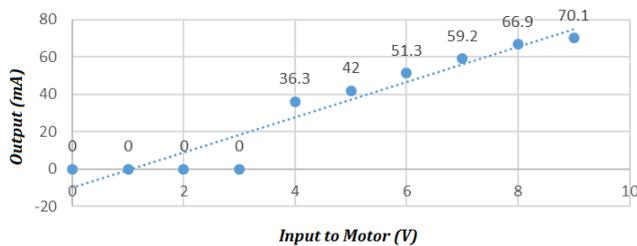
Fig. 12: JGB37-3530 testing with load
