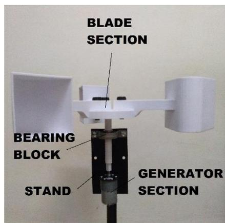
Fig. 9: HAWT prototype
