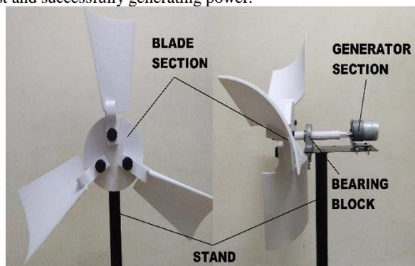
Fig. 8: VAWT prototype
