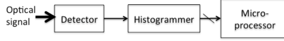
Fig. 5. Receiver block diagram for a direct detection photon counting pulsed modulation IPDA lidar.
