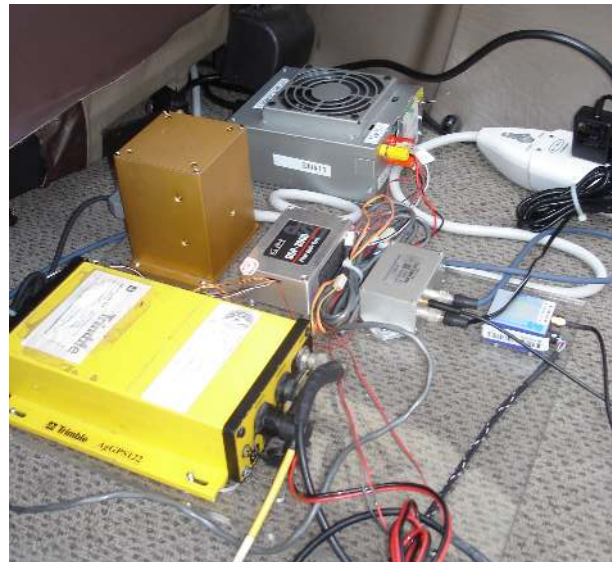
Fig. 1. Navigation Sensors installed in the cargo area of a Cessna 172
