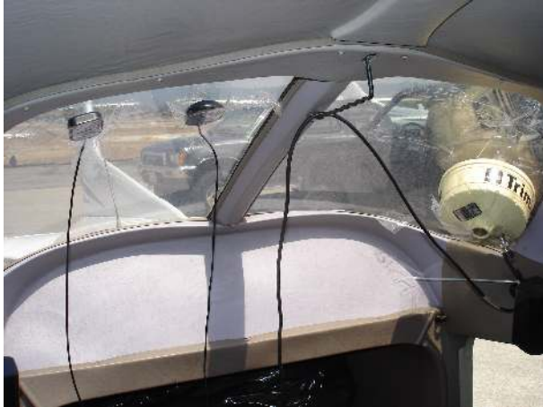
Fig. 2. GPS antenna affixed to the rear window of the aircraft
