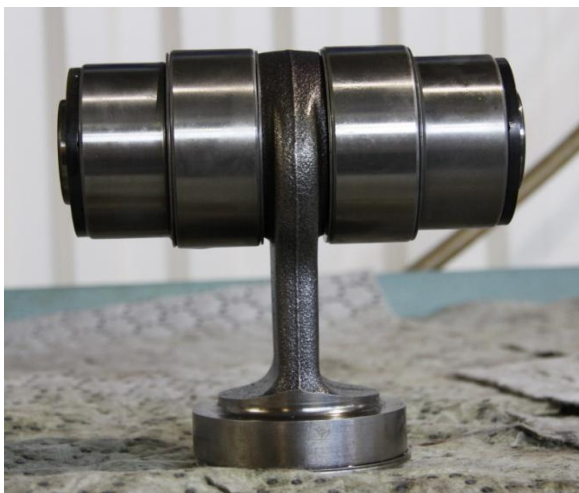
Figure 3: Actual piston assembly consisting of piston, cross pin and bearings.
