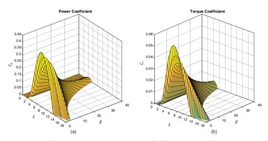
**Figure 13.** Coefficient proposed by Khajuria and Kaur [32], with variations of  $\lambda$  and  $\beta$ ; (**a**) power coefficient, (**b**) torque coefficient.
