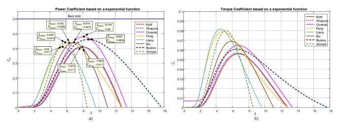
**Figure 11.** Coefficients based on an exponential function; (**a**) power coefficient, (**b**) torque coefficient. Kotti [30,31], Khajuria [32], Ov ando [33–41], Feng [42–47], Llano [48], Shi [19,50], Bustos [51], Ahmed [52].
