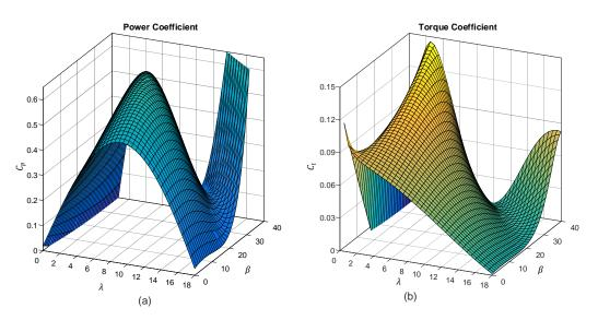
**Figure 7.** Coefficient proposed by Moussa, Bouallegue, and Kehedher [19], with variations of  $\lambda$  and  $\beta$ ; (**a**) power coefficient, (**b**) torque coefficient.
