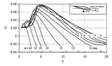
**Figure 4.** Torque coefficient for a specific type of turbine, with variations of  $\lambda$  and  $\beta$ .
