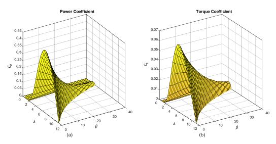
**Figure 17.** Coefficient proposed by Shi, Zhu, Cai, Wang, and Yao [49,50], with variations of  $\lambda$  and  $\beta$ ; (a) power coefficient, (b) torque coefficient.
