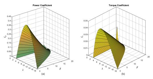
**Figure 8.** Coefficient proposed by Xin, Wanli, Bin, and Pengcheng [28], with variations of  $\lambda$  and  $\beta$ ; (a) power coefficient, (b) torque coefficient.
