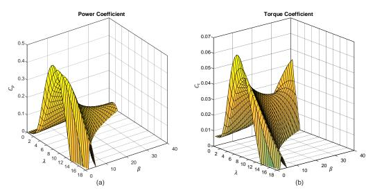
**Figure 14.** Coefficient proposed by Ovando, Aguayo, and Cotorogea [33–41], with variations of  $\lambda$  and  $\beta$ ; (**a**) power coefficient, (**b**) torque coefficient.
