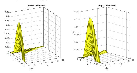
**Figure 12.** Coefficient proposed by Kotti, Janakiraman, and Shireen [30], with variations of  $\lambda$  and  $\beta$ ; (a) power coefficient, (b) torque coefficient.
