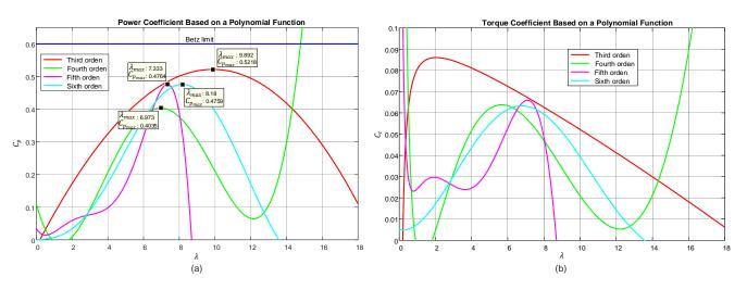
Figure 5. Coefficients based on a polynomial function; (a) power coefficient, (b) torque coefficient.
