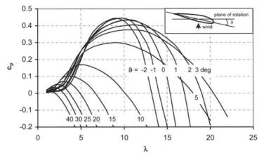
**Figure 2.** A power coefficient for a specific type of turbine, with variations of  $\lambda$  and  $\beta$  [17].
