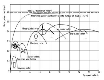
**Figure 1.** A power coefficient that depends on  $\lambda$  and the type of wind turbine [17].
