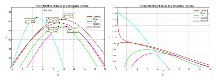
**Figure 6.** Coefficient based on a sinusoidal function; (**a**) power coefficient, (**b**) torque coefficient. Moussa [19], Coto [27], Xin [28], Merahi [29] and Nouira [18].
