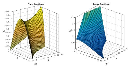
**Figure 10.** Coefficient proposed by Nouira and Khedher [18], with variations of  $\lambda$  and  $\beta$ ; (**a**) power coefficient, (**b**) torque coefficient.
