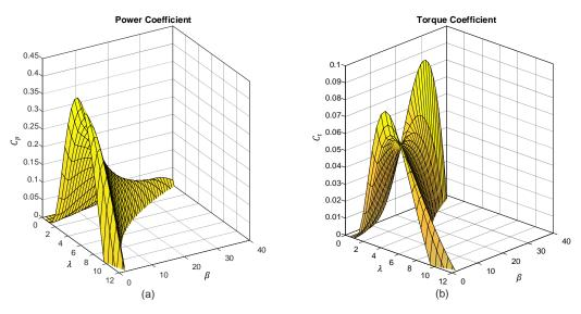
**Figure 16.** Coefficient proposed by Llano, Tatlow, and McMahon [48], with variations of  $\lambda$  and  $\beta$ ; (a) power coefficient, (b) torque coefficient.
