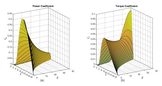
**Figure 18.** Coefficient proposed by Bustos, Vargas, Milla, Saez, Zareipour, and Nuñez [51], with variations of  $\lambda$  and  $\beta$ ; (**a**) power coefficient, (**b**) torque coefficient.
