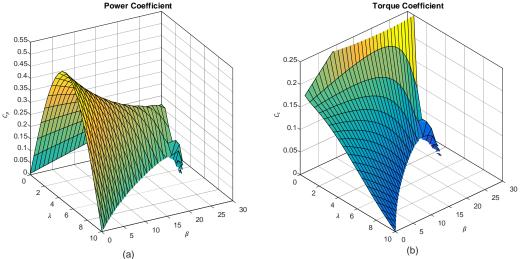
**Figure 9.** Coefficient proposed by Merahi, Mekhilef, and Madjid [29], with variations of  $\lambda$  and  $\beta$ ; (a) power coefficient, (b) torque coefficient.
