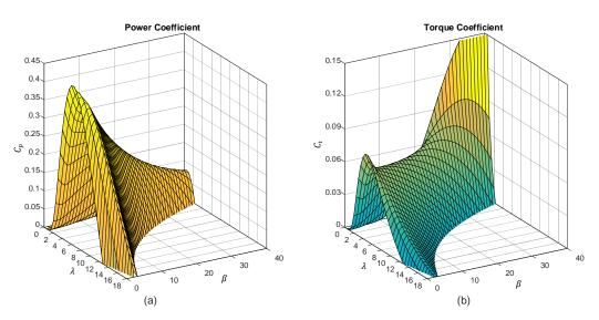
**Figure 15.** Coefficient proposed by Feng Gao, Da-Ping Xui, and Yue-Gang Lv [42–47], with variations of  $\lambda$  and  $\beta$ ; (**a**) power coefficient, (**b**) torque coefficient.
