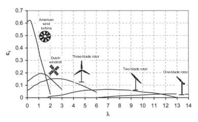
**Figure 3.** Torque coefficient that depends on  $\lambda$  and the type of wind turbine [17].
