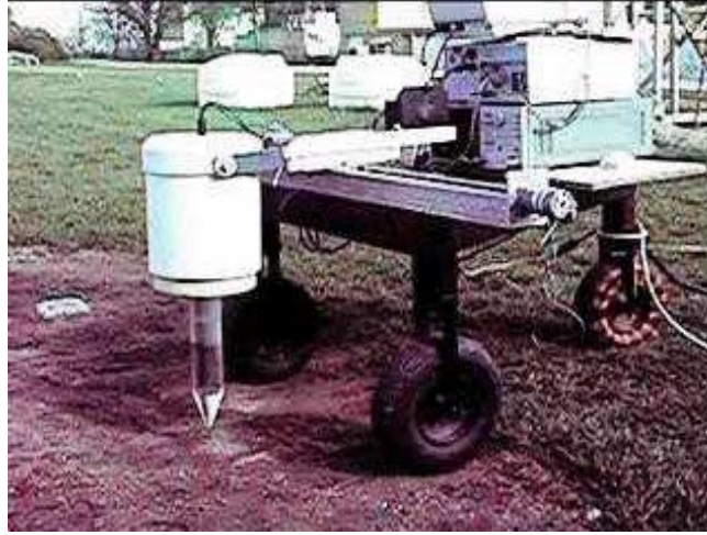
Figure 1. The GPR dielectric rod antenna and scanning system.
