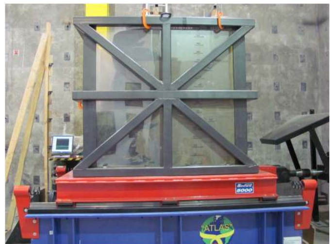
Fig. 1. Shake table test of seismic responses of MSE walls
