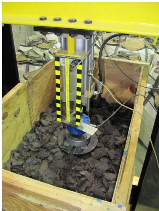
Fig. 3. Experimental setup of TDA compression test
