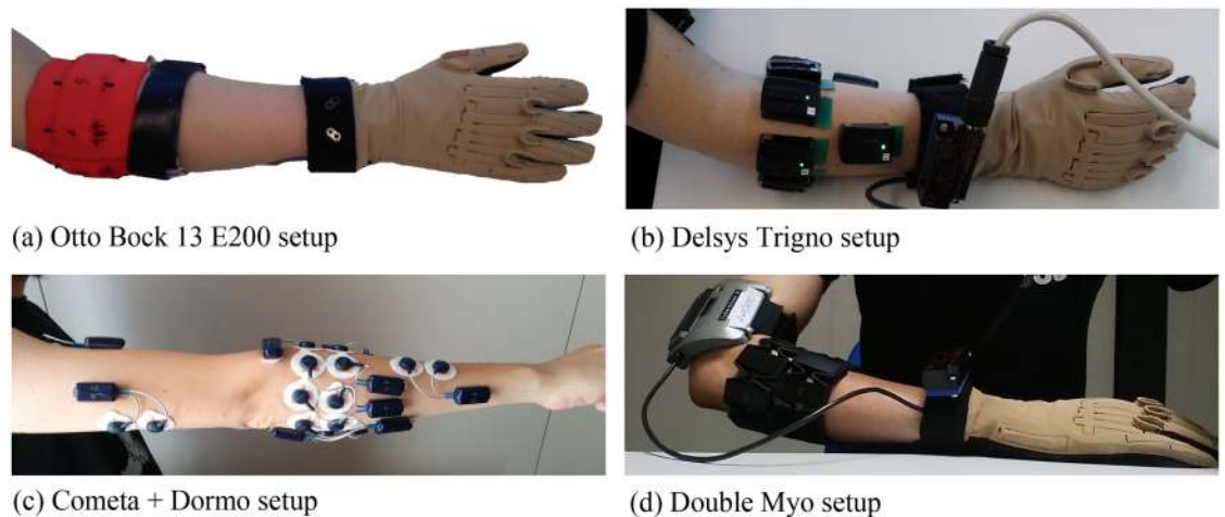
Fig 1. Acquisition setups for DB1 Otto Bock 13E200 (a), DB2 Delsys Trigno (b), DB4 (Cometa+Dormo) (c) and DB5 (Double Myo) (d).
