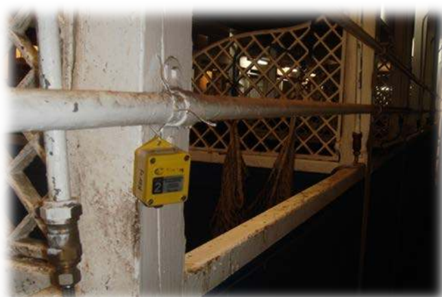
Figure 2. Placement of a data logger in one of the four stables in the study. This particular data logger was placed at the head of a tie stall at the height of the horse's breathing zone.
