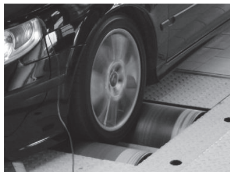
Figure 2. Cylindrical test room.
